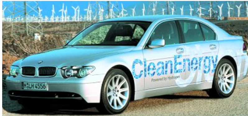
BMW's expensive 7 Series hydrogen car carries hydrogen gas on board and requires special hydrogen filling stations
